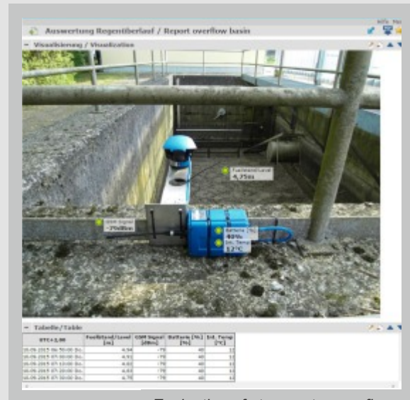
Evaluation of stormwater overflow
