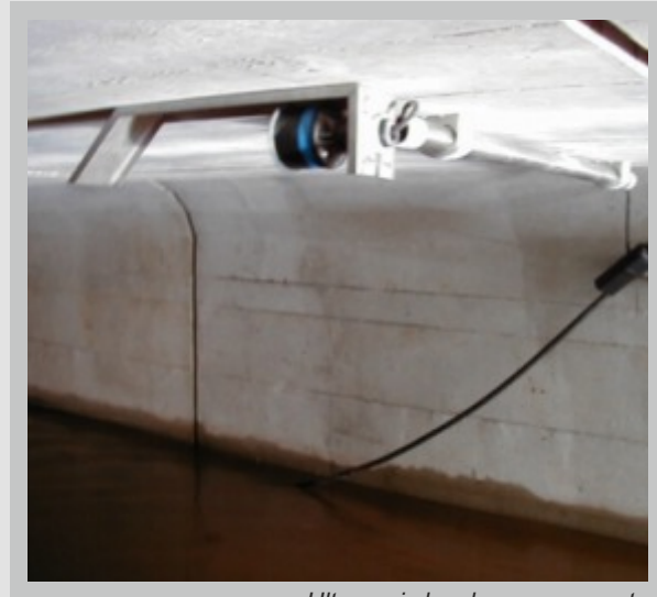
Ultrasonic level measurement with tilted mirror
